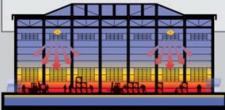
INFRARED TWO-STAGE HEATING SYSTEM
